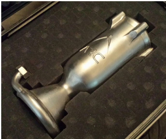
A prototype of one of ARC's engines that was tested and designed using HPC simulations and produced by additive manufacturing.
