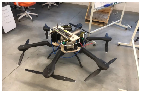
Pictured: Amogy ammonia-powered battery solution onboard a drone
